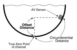
Figure 3-3 Zero Level Offset Measurement
